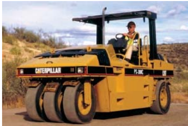
Figure 33: Caterpillar PS/PF-360C pneumatic-tire compactor (from product brochure Sept., 2004)
