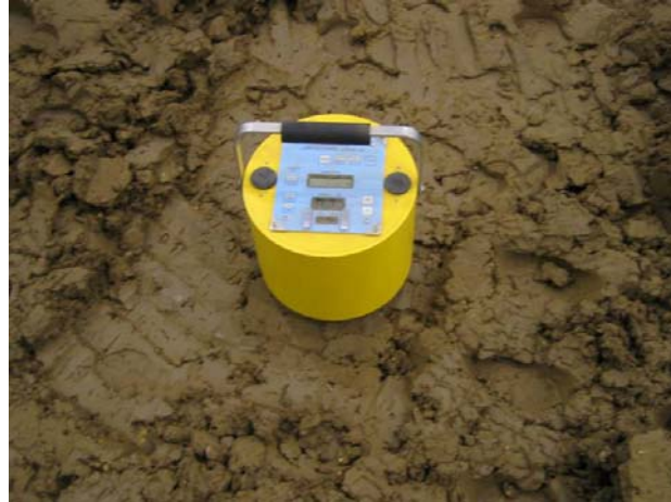
Figure 65: Modulus determination using soil stiffness gauge
