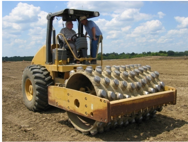
Figure 39: Caterpillar CP-533E padfoot roller
