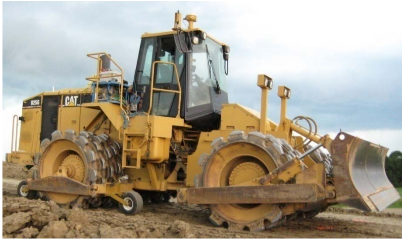
Figure 40: Caterpillar 825G tamping foot roller
