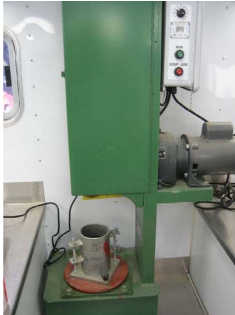
Figure 60: Automated mechanical rammer for impact compaction test
