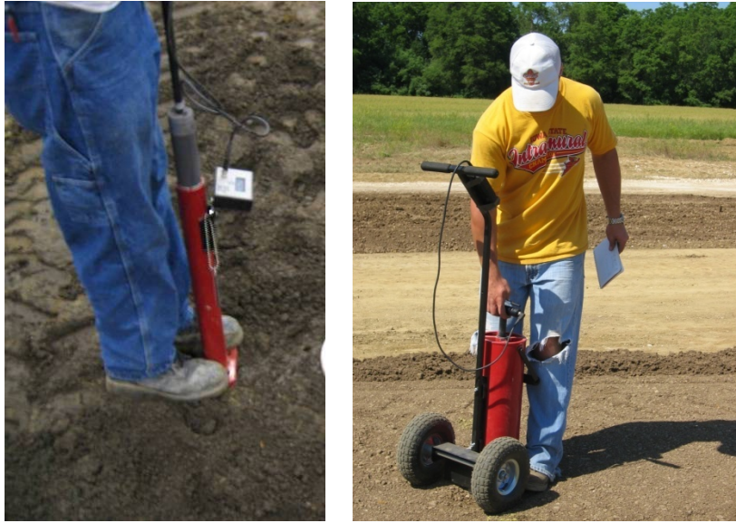
Figure 63: Strength determination using Clegg Impaction testers: 4.5-kg (left) and 20-kg (right)
